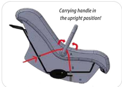
Secure the rubber bands on both sides. Closed side of the hook facing inwards. Front hook attached to lower rod!
